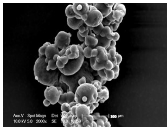
Fig. 1: SEM image of KTM microsphere
